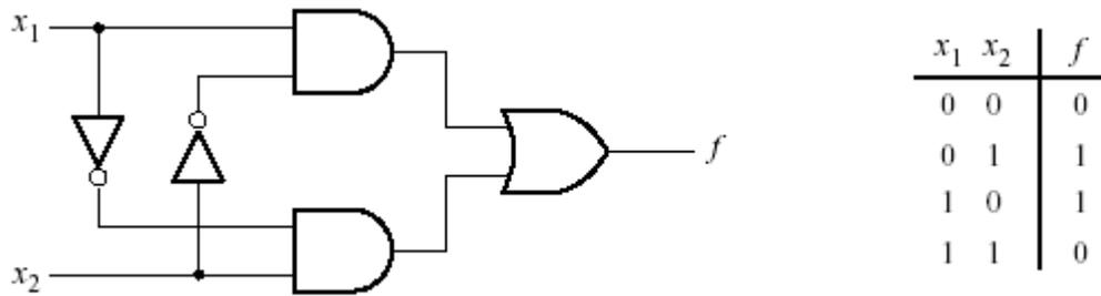
Figure 9. The light controller circuit.
