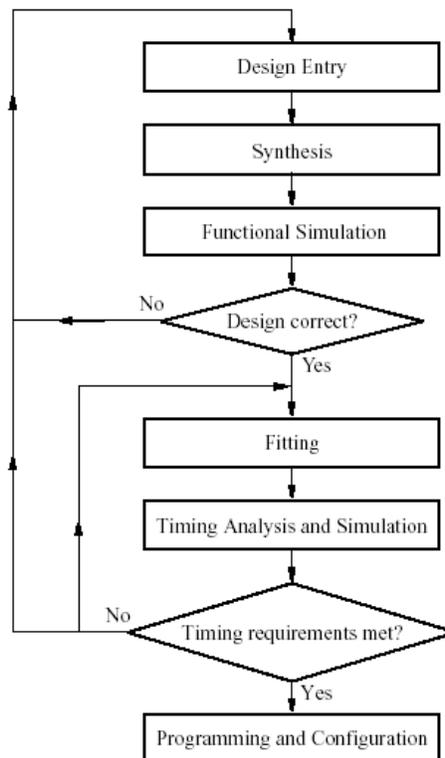
Figure 1: A typical CAD flow
