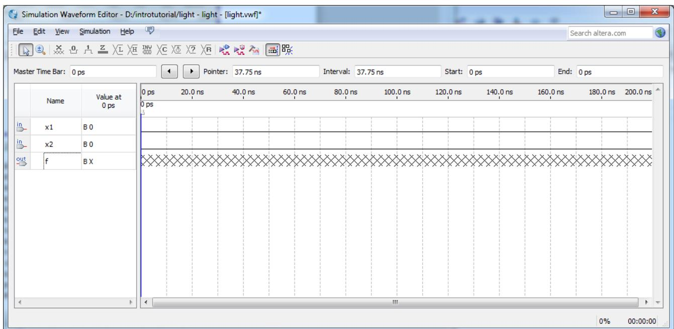
Figure 28. The nodes needed for simulation.
