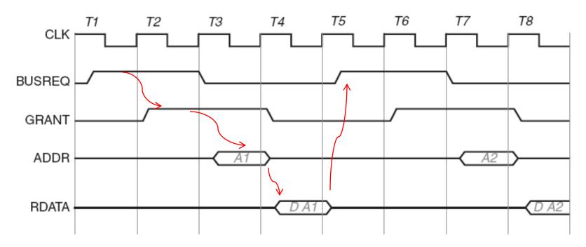
Pipelined Transfer - Overlap address and data phases Only works if separate address & data busses are present
