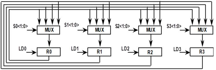
Modules have edge-triggered N-bit registers to transfer, controlled by LDi signals.
