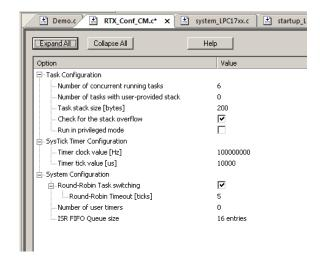
**Tip:** Any changes you make here will be reflected in the code in the Text Editor tab and vice versa. You must rebuild your files in order for any changes to have effect.
