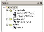
15. Click on Project/Manager and select Components, Environment.... And the window below opens up. This is where you can manage your project structure. You can add and delete Targets, Groups and files as desired. Click on OK to return to the main menu.
