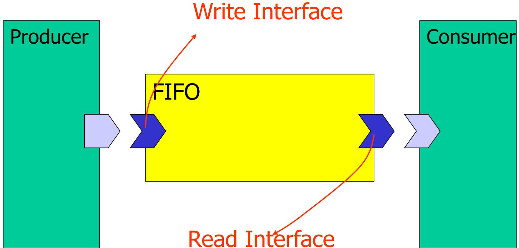
**Problem definition: FIFO communication channel with blocking read and write operation**
