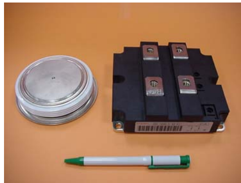
4500V/800A press pack and 1700V/1200A module diodes
