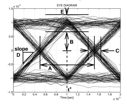
C.2 Key parameters to be measured with an eye diagram are shown below.
