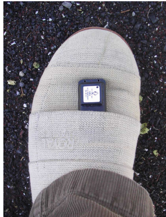
Fig. 11. Sensor module mounted on a shoe.
