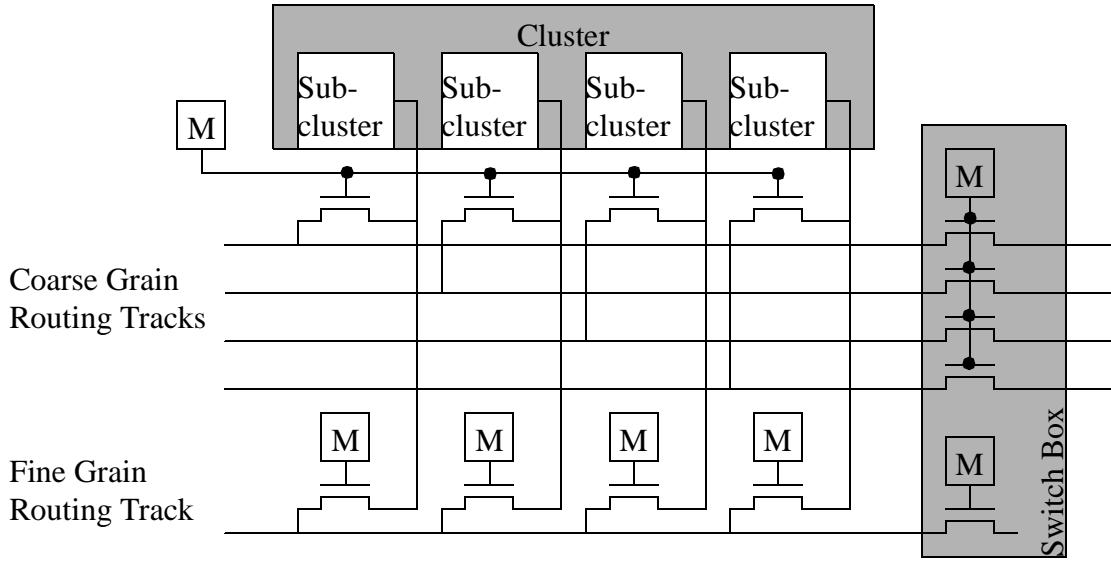
**Figure 4: Coarse Grain Routing**
