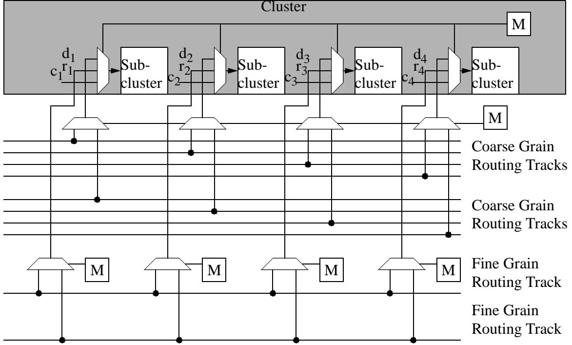
$d_1, d_2, d_3, d_4$  — datapath input connections from coarse grain routing buses
