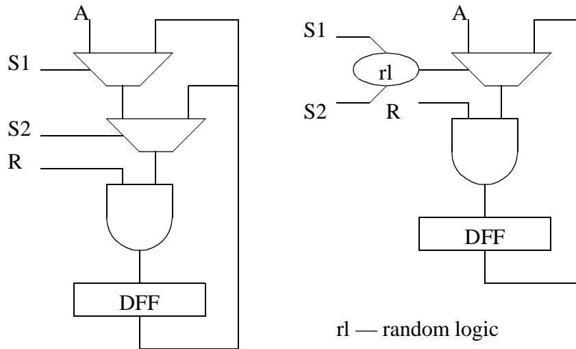
**Figure 9: Mux Tree Collapsing Example**
