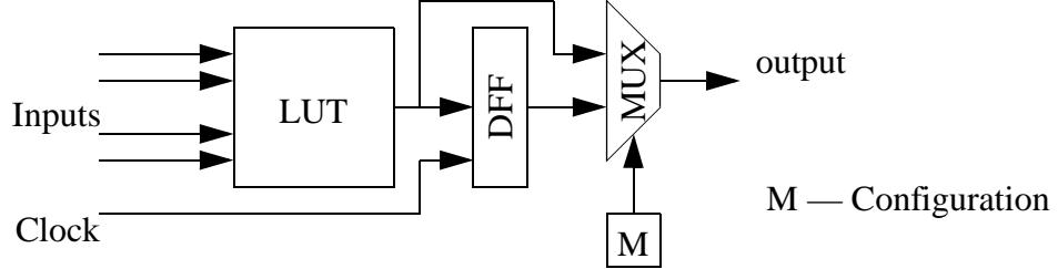
**Figure 1: A Basic Logic Element (BLE)**
