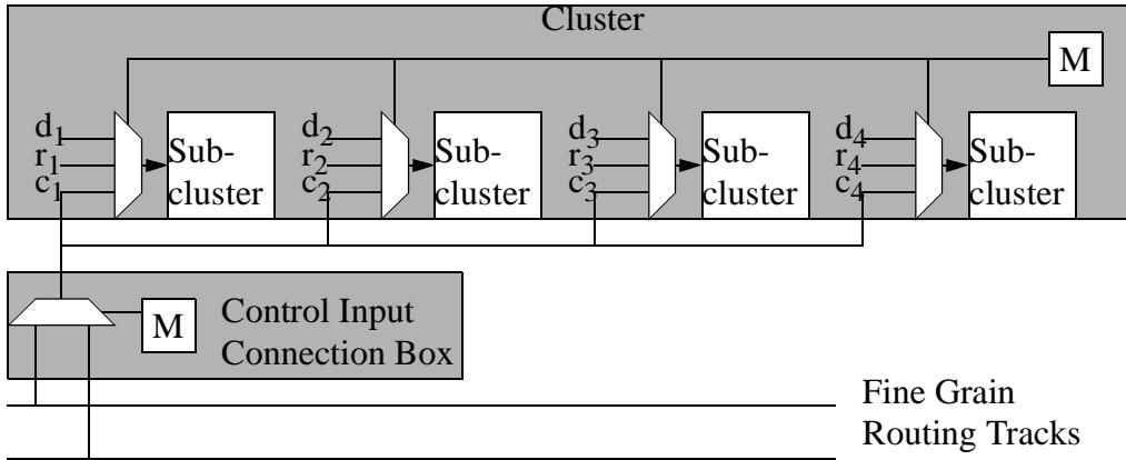
$d_1, d_2, d_3, d_4$  — datapath input connections from coarse grain routing buses
