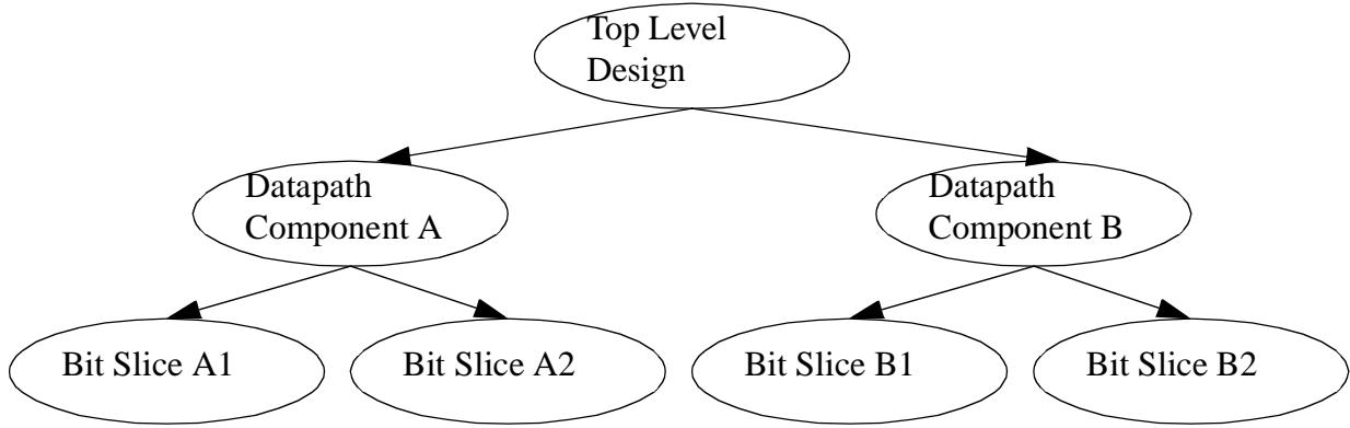
**Figure 8: Hierarchical Structural of the Initial Synopsys Compile Output**
