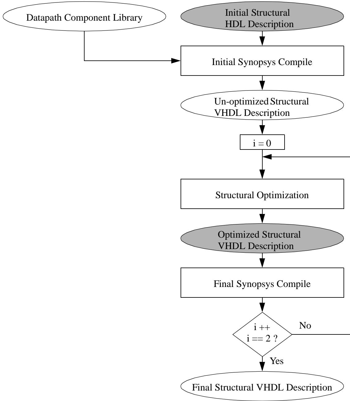
**Figure 7: Overall Flow of the Synthesis Tool**
