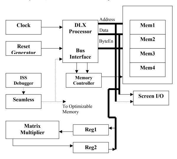
Figure 1 DLX Architecture with Matrix Multiplier
