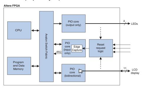
Figure 11-1. An Example System Using Multiple PIO Cores
