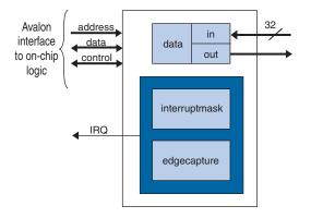
Figure 11–3 shows a block diagram of the PIO core configured in bidirectional mode, without support for IRQs.
