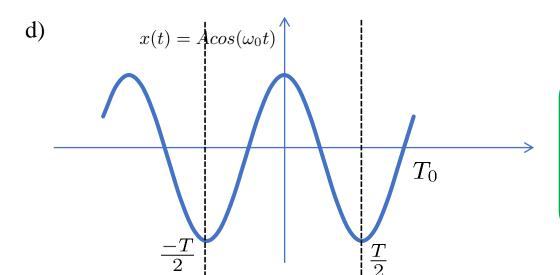
For periodic signals with fundamental period  $T_0$  we have
