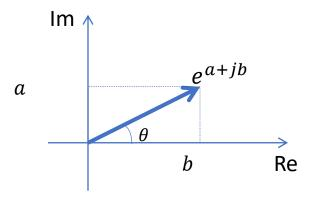
$$|e^{st}|^2 = |e^{\sigma t}e^{j\omega t}|^2 = |e^{\sigma t}|\underbrace{|e^{j\omega t}|^2}_1 = e^{2\sigma t}$$
