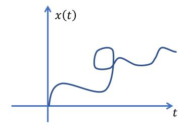
**Answer:** The above graph is NOT a signal. For the function x(t) to be a signal, there must be no more than one value of x(t) at any given time t.
