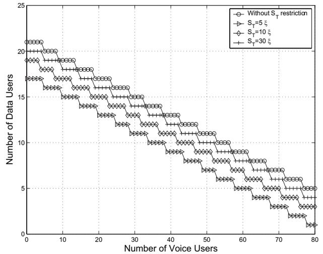
Fig. 3. Capacity curves for cases with and without sum power constraint.
