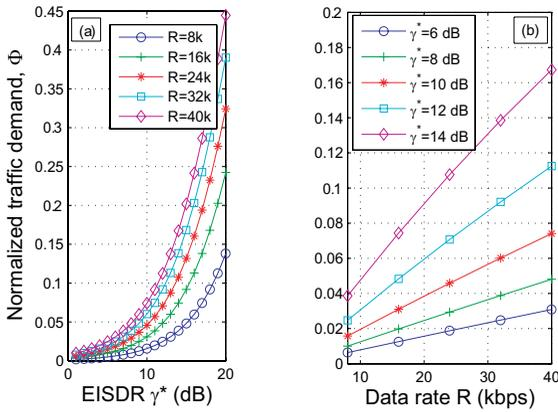
Fig. 1. Normalized traffic demand as a function of the QoS requirements.
